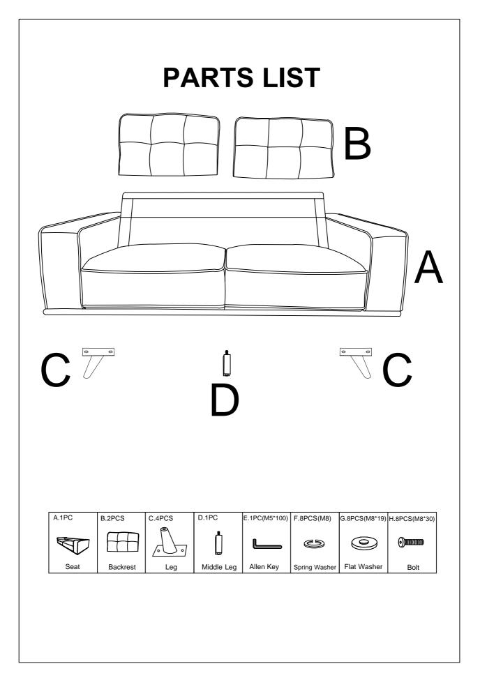
Attach leg(C) to base frame(A) ,using bolt(H) with flat washer(G) and spring washer(F),then fasten by allen key(E). Attach middle leg (D) by fastening to thread in centre of base. With 2 people carefully turn over
